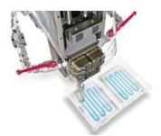
Heat-conducting media with a viscosity of up to 1,000,000 mPa·s can be applied quickly and precisely with the newly developed high-performance dispenser Dos HP.
