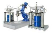
The new system solution for battery encapsulation, consisting of the high-performance dispenser Dos HP and the material feeding unit PailFeed200 Abrasive, offers dispensing speeds of up to 80 ml/s even when using highly abrasive thermally conductive media.
